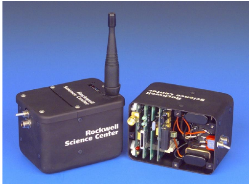
Fig. 1. WINS Sensor Node from RSC
